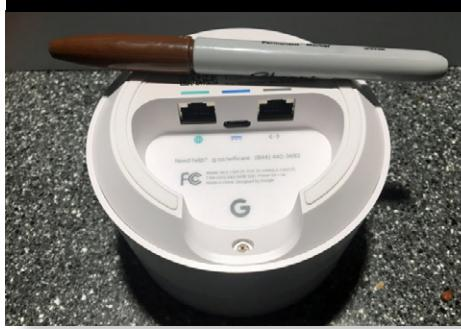
The bottom of the Google Wifi unit has Ethernet ports
