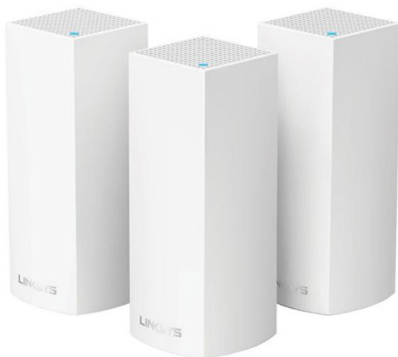
The Linksys Velop whole-home Wi-Fi system comes with three identical nodes. After connecting the first node to a broadband modem, the other two create a wireless mesh network.
