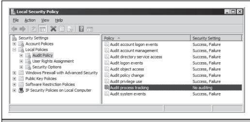
**Figure 4-1** Recommended audit settings for a secure server, as configured using Windows Server 2008's Security Policy snap-in
