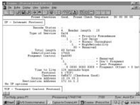
Figure 14-7 Pogo's policy route has set the Precedence bits of this packet to priority (001b) and the TOS bits to minimum delay and maximum reliability (1010b).
