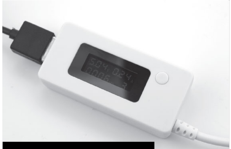
Figure 1: A USB power meter, reading the power flowing into a Raspberry Pi 2
