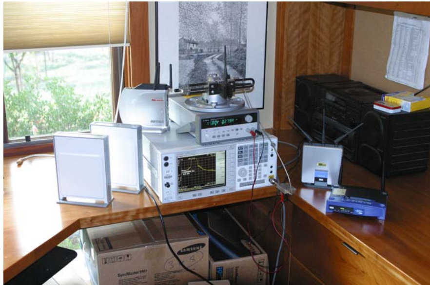
Figure 2 - The spectrum analyzer (an Agilent E4443A) used to monitor air conditions, as well as the five routers tested. Source: Farpoint Group.
